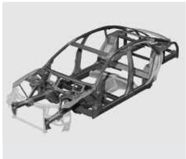
Aluminium Space Frame (ASF) as the supporting structure for an all-aluminium body of a production series car
