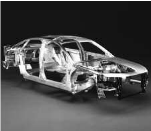
Aluminium Space Frame (ASF) as the supporting structure for an all-aluminium body of a production series car
