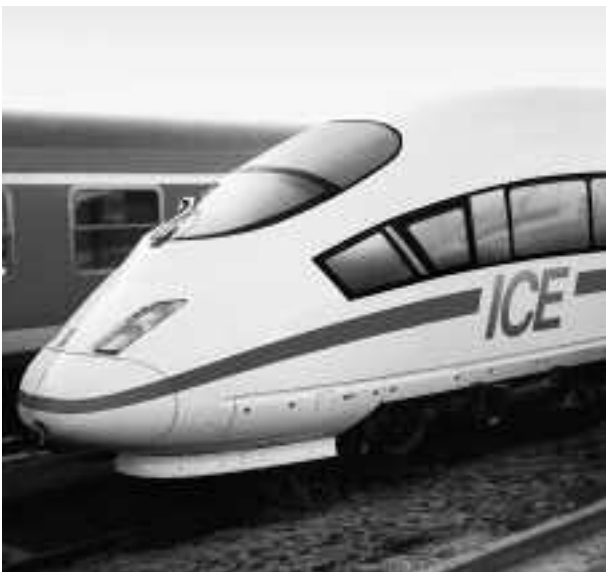
The middle carriages of the ICE train are made from welded extruded aluminium profiles up to 800 mm wide and over 23 m long
